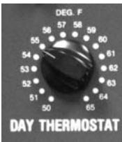
The Day Thermostat Dial should be set at the outdoor temperature above which no heat is required. When the outdoor temperature is below the setting of this dial the amount of heat provided each hour will be regulated by the Heat-Timer and will be proportional to the weather and the specific heat requirements of the building.
