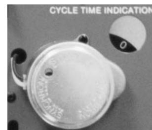
The -60 model total cycling time is one hour. The heat "on" portion is determined by the outdoor temperature. The colder the weather, the longer will be the "on" portion of the cycle. The "off" portion of the cycle is the difference between the "on" portion and one hour. For example, if the "on" portion is 32 minutes, the "off" portion will be 28 minutes.
