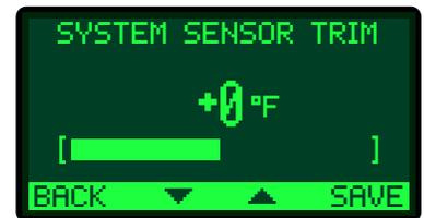
Do not use the Trim setting to make the Outdoor temperature sensor match the temperature reported on the radio or TV. Outdoor temperatures can vary widely over a broadcast range. Only trim the outdoor sensor based on accurate thermometer reading taken where the sensor is located.
