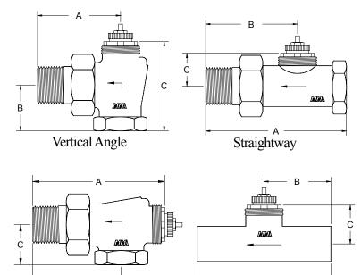
Macon NT Series Valves are in an open position when no operator is attached.
