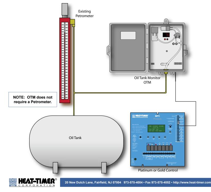
The Oil Tank Monitor has a pump for automatic pressure compensation. An internal timer energizes the pump at regular intervals to insure correct operation. The pump can also be programmed to activate immediately for testing or after maintenance.
