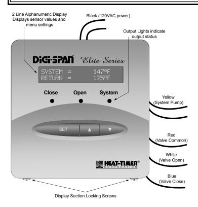
The RSM-Elite is designed to control under slab heating systems to prevent accumulations of ice or snow. To do this, it monitors three temperatures, the outside temperature, the temperature of the fluid going to the slab, and the temperature of the fluid returning from the slab.
