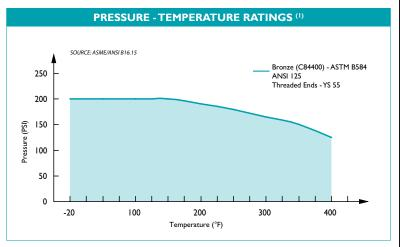
I. The pressure-temperature ratings given are ONLY for the YS 55-BZ (Threaded) per ASME B16.15. The internal working pressure rating for a solder joint strainer is dependent, not only on the strainer, but also on the composition of the solder used for the joint. The working pressure ratings shown for model YS 56-BZ (Solder) are representative of using an alloy Sb5 95-5 tin-antimony solder. For other solder joints, please consult factory.
